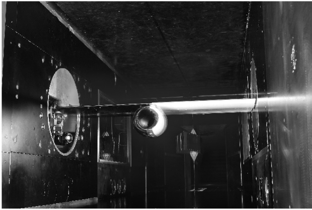
Fig. 1 Photograph of the WIONA model mounted in the adaptive test section of the DNW-TWG wind tunnel.
